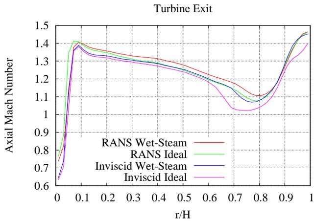
**FIGURE 18.** ABSOLUTE AXIAL MACH NUMBER AT TURBINE EXIT PREDICTED BY VARIOUS FLOW MODELS
