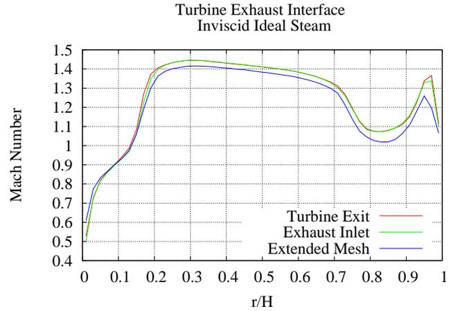
**FIGURE 4.** MACH NUMBER AT MIXING PLANE
