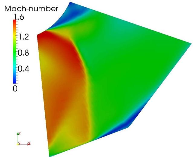
**FIGURE 20.** FLOW MACH NUMBER IN EXHAUST SECTION PREDICTED BY RANS WET-STEAM SIMULATION
