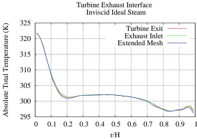
FIGURE 6. TOTAL TEMPERATURE AT MIXING PLANE
