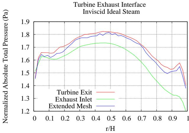
FIGURE 5. TOTAL PRESSURE AT MIXING PLANE
