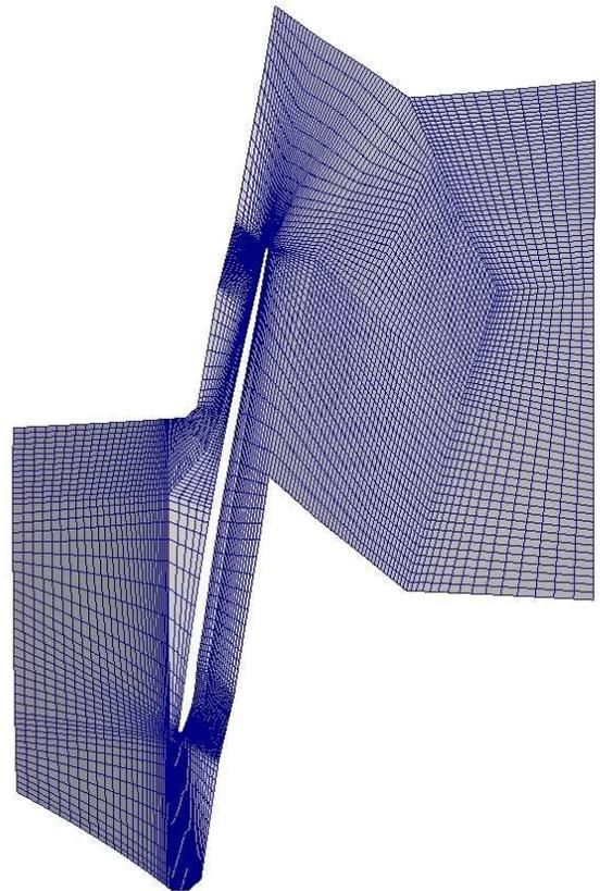
**FIGURE 14.** TURBINE MESH AT SHROUD FOR INVISCID FLOW
