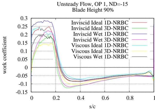
**FIGURE 23.** NORMALIZED WORK COEFFICIENT ON SUCTION SIDE AT 90% BLADE HEIGHT FOR NODAL DIAMETER -15
