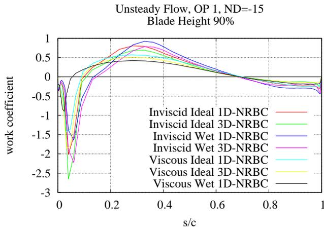
**FIGURE 22.** NORMALIZED WORK COEFFICIENT ON PRESSURE SIDE AT 90% BLADE HEIGHT FOR NODAL DIAMETER -15
