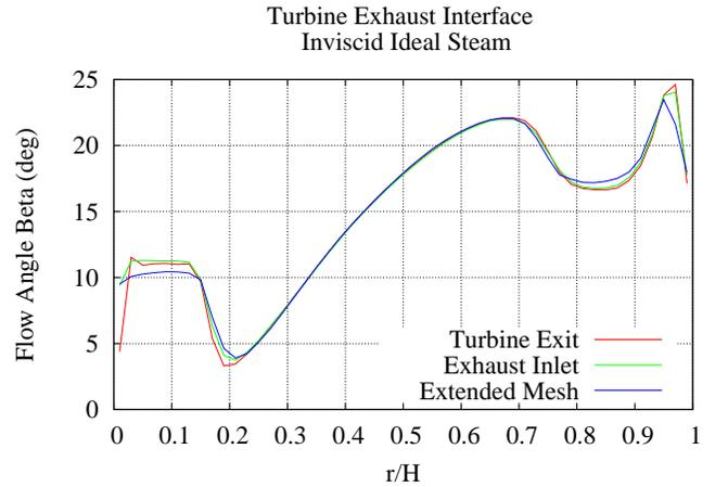
FIGURE 8. ABSOLUTE FLOW ANGLE BETA AT MIXING PLANE
