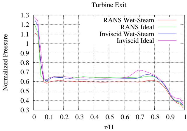
**FIGURE 19.** NORMALIZED STATIC PRESSURE AT TURBINE EXIT PREDICTED BY VARIOUS FLOW MODELS
