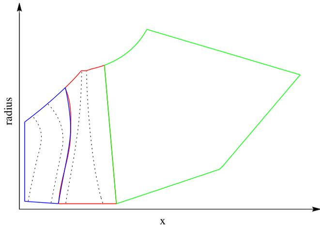
**FIGURE 15.** SCHEMATIC OF MULTI-ROW FLOW DOMAIN FOR THE NEW BLADE
