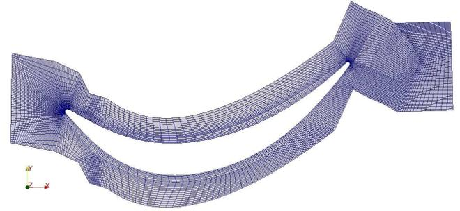
**FIGURE 13.** TURBINE MESH AT HUB FOR INVISCID FLOW
