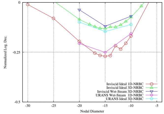
**FIGURE 24.** PLOT OF NORMALIZED LOGARITHMIC DECREMENT FOR VARIOUS FLOW MODELS
