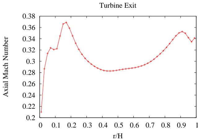
**FIGURE 9.** AXIAL MACH NUMBER AT TURBINE EXIT FOR NON-REFLECTING BOUNDARY CONDITION TEST CASE
