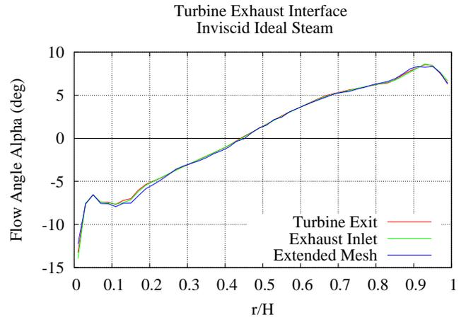
FIGURE 7. ABSOLUTE FLOW ANGLE ALPHA AT MIXING PLANE
